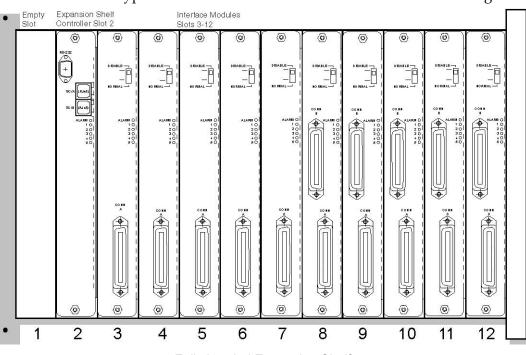
The shelf diagram below shows a fully loaded Expansion Shelf. Any type of Interface Module can be installed in slots 3 through 12.
